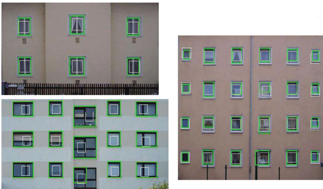
Figure 8: Additional results – Hypotheses (white squares) and windows (green rectangles) for buildings from Bonn and Munich
